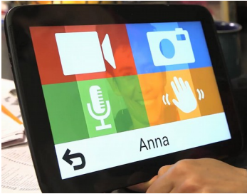
Figure 1: InTouch is an accessible communication app supports asynchronous communication with loved ones: sending/receiving of images, audio, or video, receiving (but not sending) text messages, and sending of one pre-defined “I’m thinking of you” message. It has a non-language specific interface (based on icons), and requires no typing because it was also developed for seniors with dexterity problems or related motor impairments.
